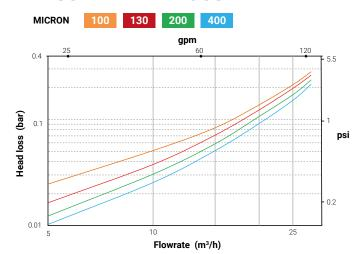
\*The backwash frequency depends on the design flowrate. For hydraulic calculation, consider the set-point value for the self-cleaning cycle (usually 0.5 bar/7.25 psi).
